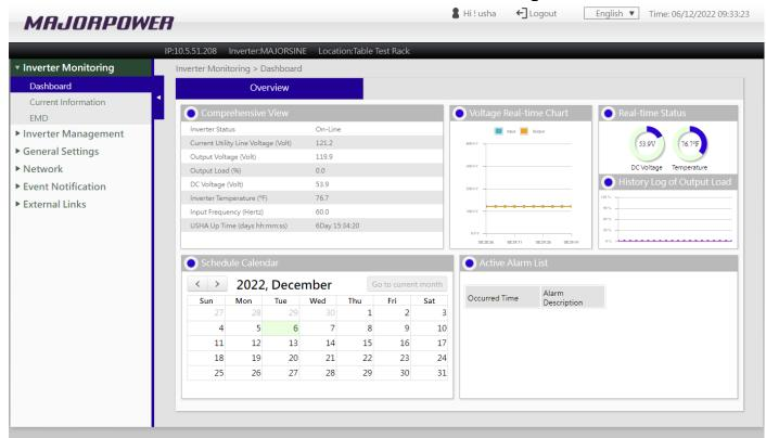
In a Dashboard Current Status page, one can check the operating status, schedule, and parameters of the inverter. This page will refresh automatically with the real time operating status of the inverter, schedule, alarm and equipment information.
