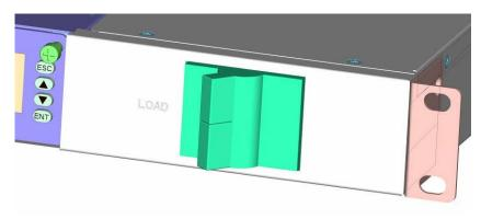
This power system is designed with the integrated output circuit-breaker 2-Pole interrupt, front access operation. The two pole power block for secured screw connections is located on the system backside. The circuit breaker separates both the positive and negative circuits between the system output
