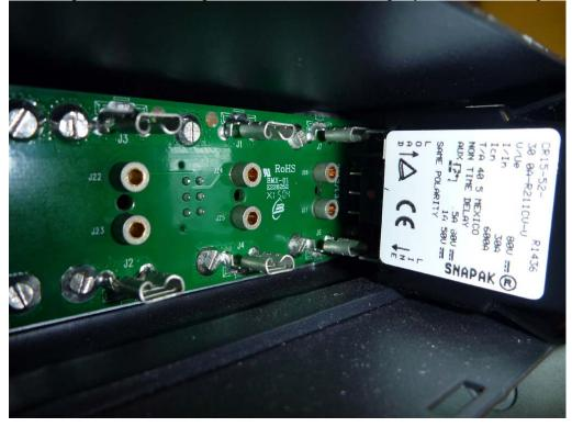
★ Each set of female terminals may need to be adjusted to properly align with and receive the breaker. ★
